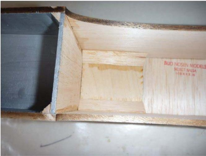
Cut some triangle stock to brace the landing gear block.
