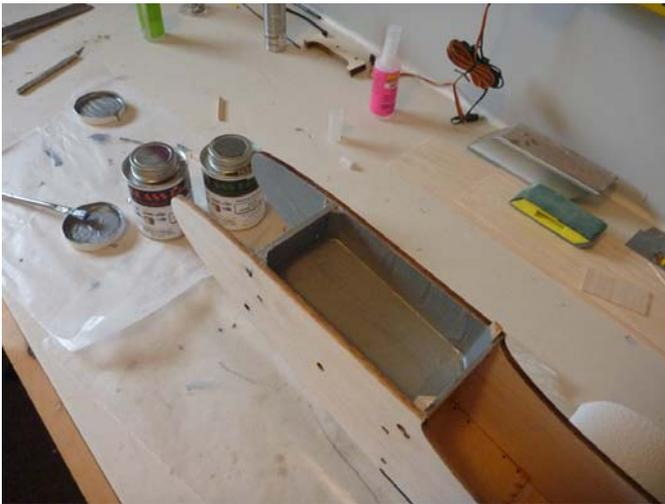
Take this time to fuel proof the engine and tank area. Use CA or epoxy.
