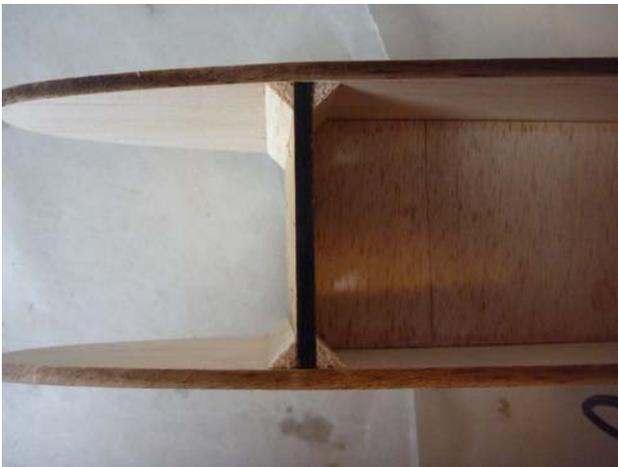
Cut some triangle stock to size for the fire wall. Glue the triangle stock on both sides, on top and under the fuel tank floor. Also, not shown here glue some triangle stock to the bulkhead at the front of the wing on the fuel tank side.
