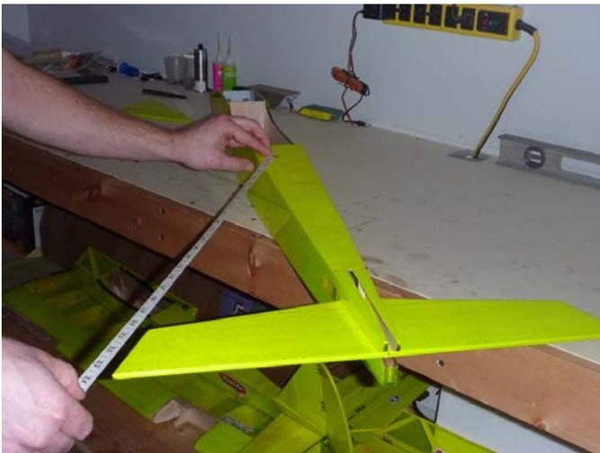
Line up the horizontal stab and vertical stab. When in their place, mark and remove covering where gluing. Glue vertical and horizontal stab at the same time. Take your time on this step. Next install the elevator and the rudder. There are predrilled holes if you wish to hinge by the sewing method, or you can use conventional hinges if you desire.
