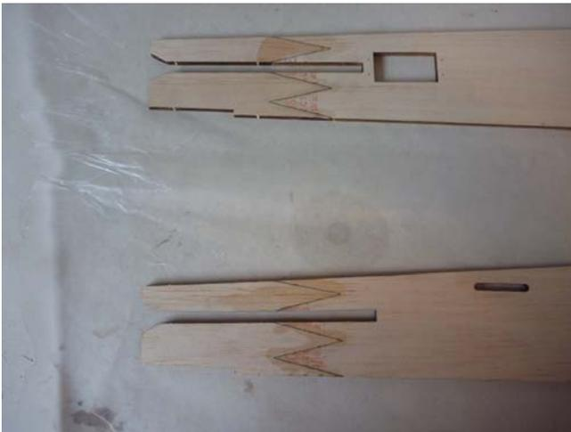
Start with the fuselage sides and glue the back pieces on. Put the fuselage sides aside.
