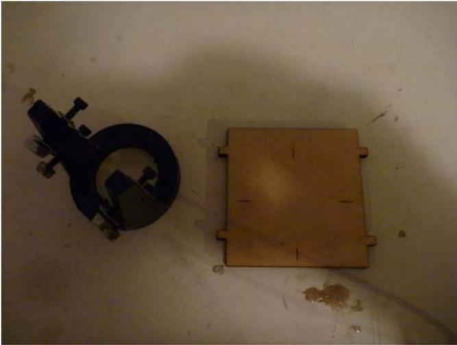
If you have decided to use the firewall with the holes not pre drilled now is a good time to do it your self. Use the vertical and horizontal marks to center your engine mount.
