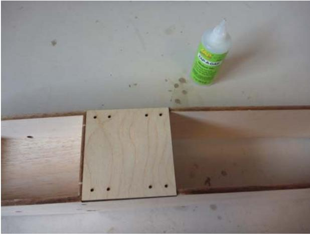
Next install the landing gear mount making sure it is flush with the fuselage sides.
