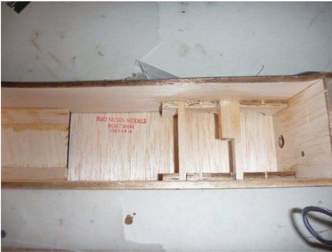
Check the servo mounts to make sure the slots cut out are the right size for your intended servo. It may be necessary to make the slots a little larger to fit your servo.
