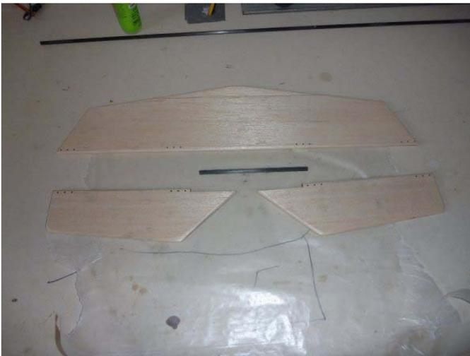
Cut a piece of  $\frac{1}{4}$ " dowel hard wood or carbon fiber to size for the elevators. Sand the dowel so the glue will adhere better. Glue with medium CA
