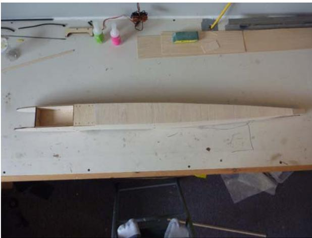
With 1/16" sheeting. Sheet the bottom of the fuselage from the landing gear block to the tail wheel mount.
